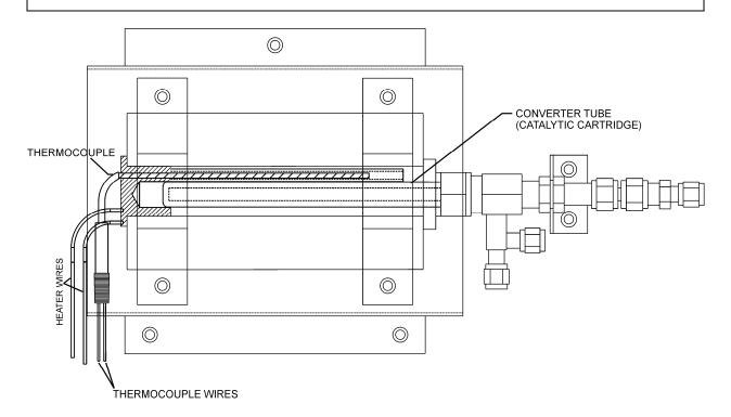
Figure 4-2. Thermocouple Location
